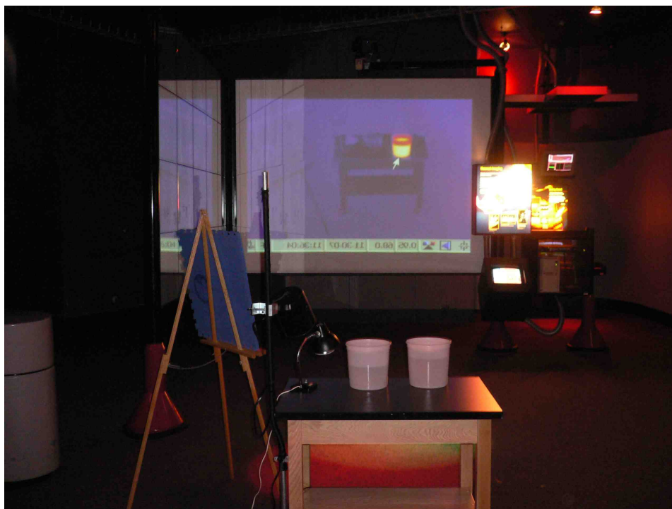
Figure 1: Setup of the materials used during the evaluation. Left to Right on the Bottom: Easel, Light, Cold Water Bucket, Hot Water Bucket. Center Top: Screen with IR image of the setup projected onto it. Note that the hot water is Yellow while the colder objects appear Blue.
