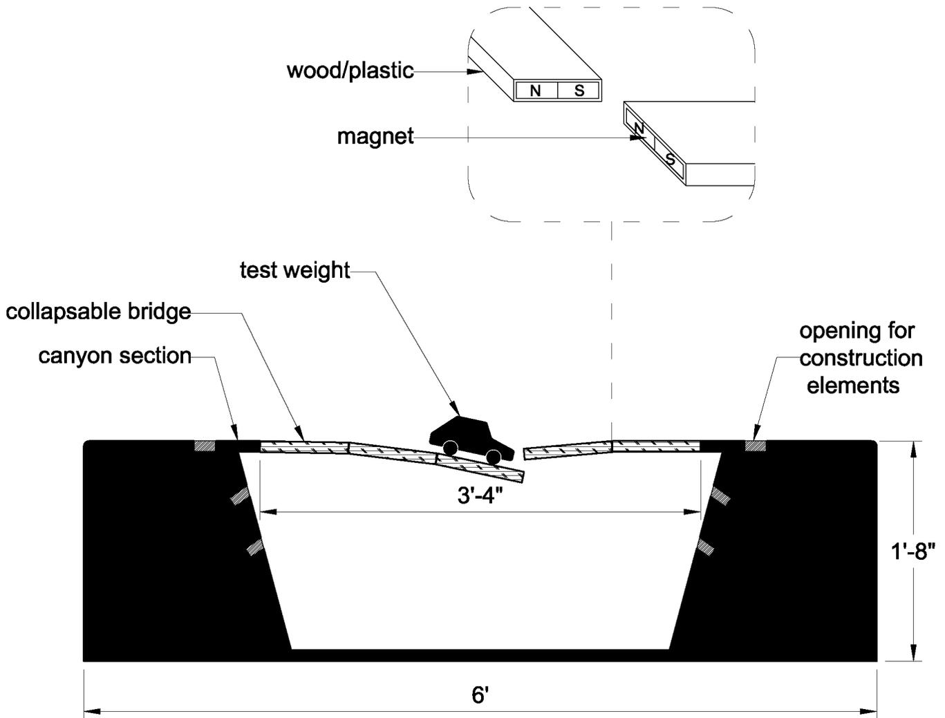
The base bridge will be self-supporting but will collapse under the weight of the car. Children need to use the separately provided wood blocks and ropes to strengthen the bridge.
