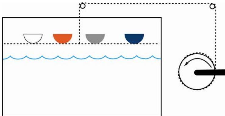
Objects may include solid materials with densities greater and less than water as well as at least one object which is made of a denser material with enclosed air spaces, either hollow or cup-shaped. A diagram above the tank identifies the different objects. A replicate set of objects is attached to exhibit but available for hands-on inspection.
