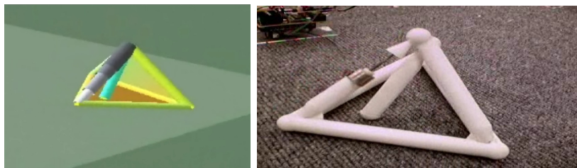
Figure 4: A sample 'evolved' walking robot. Left: Picture from program that created the robot. Right: The robot after 3D printing and installation of linear actuator.
