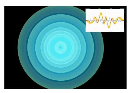
The amplitude of the sound wave is related to the distance the visitor moves the IR device. If the visitor moves the IR device a large distance the sound wave has high amplitude. The wave drawn expands to fill more space on the display, and the intensity of sound heard from the audio system increases. If the visitor moves the IR device a small distance the sound wave has low amplitude. The wave drawn shrinks on the display, and the intensity of sound heard from the audio system decreases.
